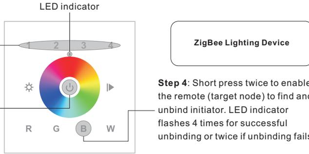
**Step 4:** Short press twice to enable the remote (target node) to find and unbind initiator. LED indicator flashes 4 times for successful unbinding or twice if unbinding fails.
