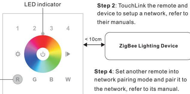
**Step 2:** TouchLink the remote and device to setup a network, refer to their manuals.
